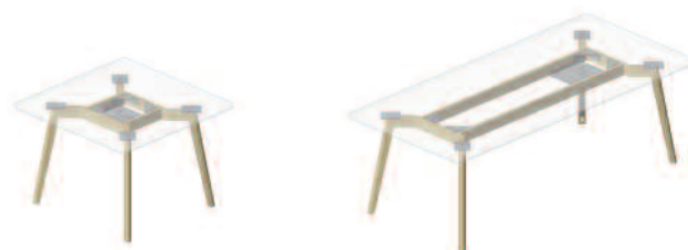
Solem table shown with wire management tray in center position on left and in end position on right. Field installed.
